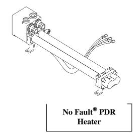
**Service Note:** The PDR Heater is used to retrofit all No Fault 6000 and Tri-Bend heaters. Some spa models may require extending the <sup>1</sup>/<sub>4</sub>" bleed line hose. <sup>1</sup>/<sub>4</sub>" vinyl tubing, one coupler, and hose clamps are provided in the service kit.
