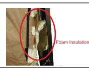
**5.** The LED Lights will be hidden behind a layer of foam and masking tape. Pry the foam and masking tape to expose the LED Light Housing. Pull the 2 LED wires straight up to separate the LED Light from the LED housing.
